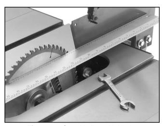
Figure 19. Guard in line with blade.
